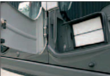
The fresh air filter for the air conditioner is relocated to the cab door side from the conventional location behind the operator seat. This allows easy cleaning and replacement of the fresh air filter, like the air circulation filter inside the cab.
