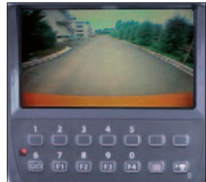
The widescreen colour LCD, in tandem with the rear view camera on the counterweight, provides a convenient view of the area behind the unit. The rear view camera automatically works when travelling backward, and can also be manually turned on with a select switch on the monitor.
