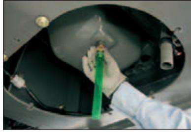
The engine oil pan is fitted with a drain coupler. When draining, an associated drain hose is connected to the drain coupler. The drain coupler is reliable, preventing oil leakage and vandalism.
